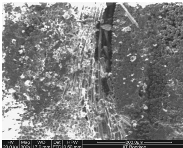
Fig. 9 SEM picture of sample B at load (20 N) sliding speed (2 m/s)
